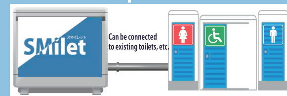
Stand-alone treatment unit
